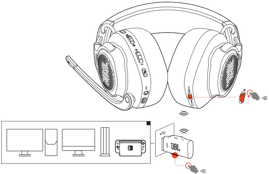
1. On the headset, slide the power switch upwards and hold for more than 5 seconds until the status LED flashes white.
