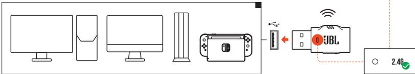
1. Plug the 2.4G USB wireless dongle into a USB-A port on your PC, Mac, PS4/PS5 or Nintendo Switch™.
