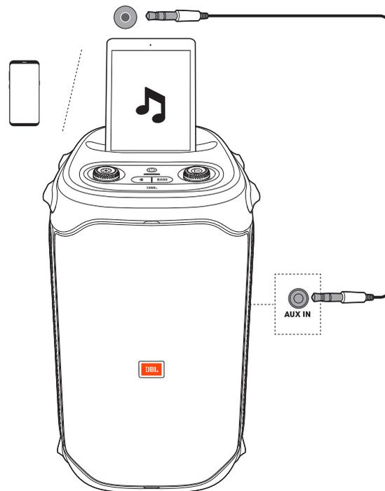
1. Connect an external audio device to the speaker through a 3.5 mm audio cable (not supplied).
