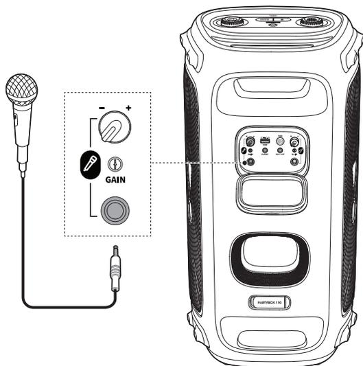
Connect a microphone to the microphone socket.
