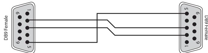
The cable is wired as a null modem:
